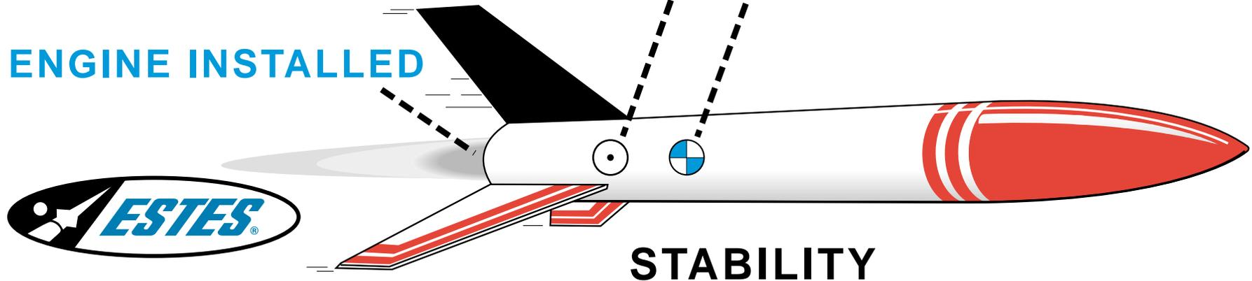
**Center of Gravity Must Be Ahead Of Center Of Pressure.
