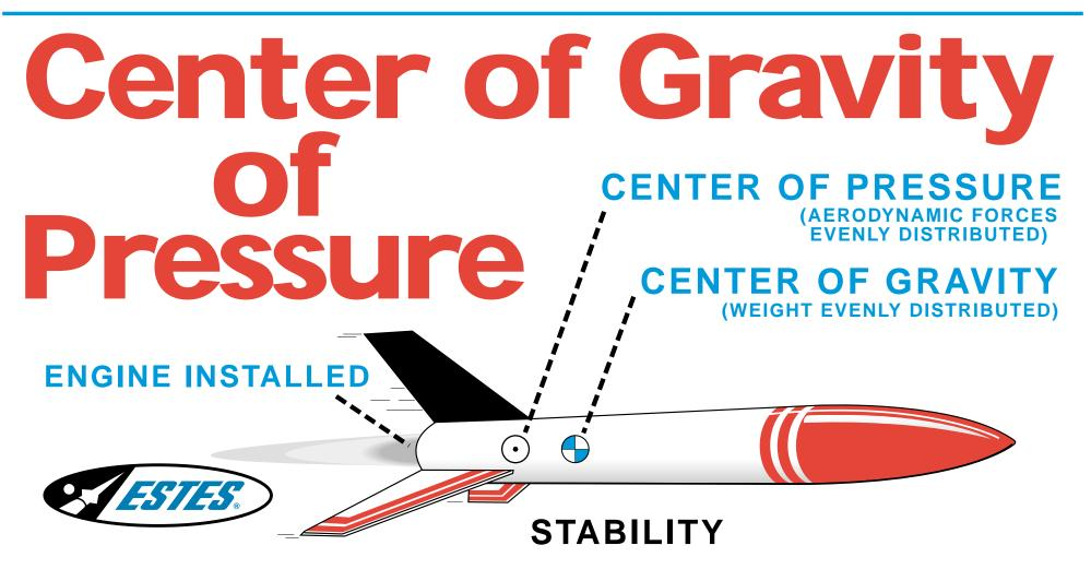
Center of Gravity Must Be Ahead Of Center Of Pressure. The Distance Between The CG And The CP Should Be Equal To Or Greater Than One Body Diameter.
